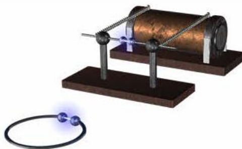
Fig. 1. The device for generating electromagnetic waves.
