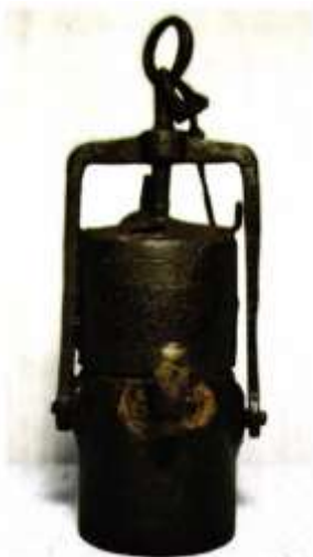
Figure 2 – Carbide lamp made of steel
