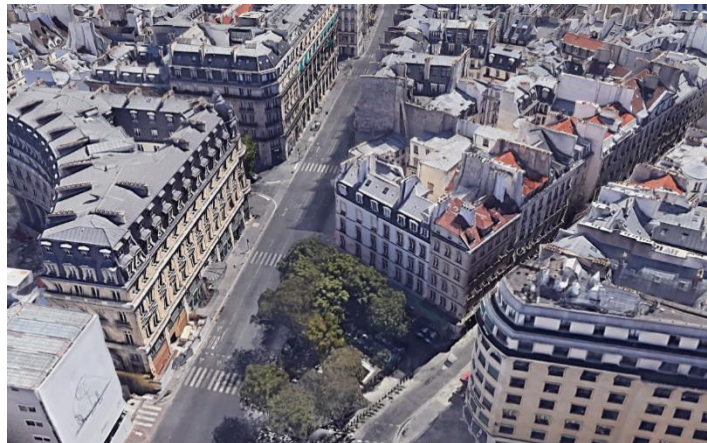
Figure 7. 3D model of the urban area obtained on the basis of the photogrammetry method
