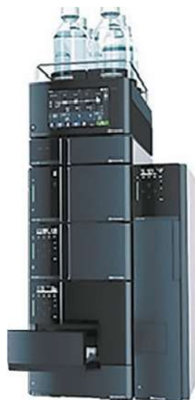
Fig. 1. Nexera LC-40 Complex for determination of aromatic hydrocarbons in oil by High Performance Liquid Chromodynamics method.
