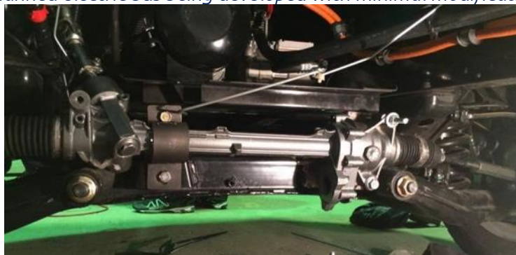
Figure 6. Electromechanical rack installed in a regular place in an electric bus
