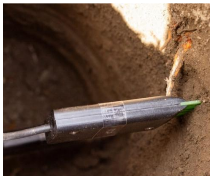
Figure 4. Time Domain Transmissometry (TDT) Sensor
