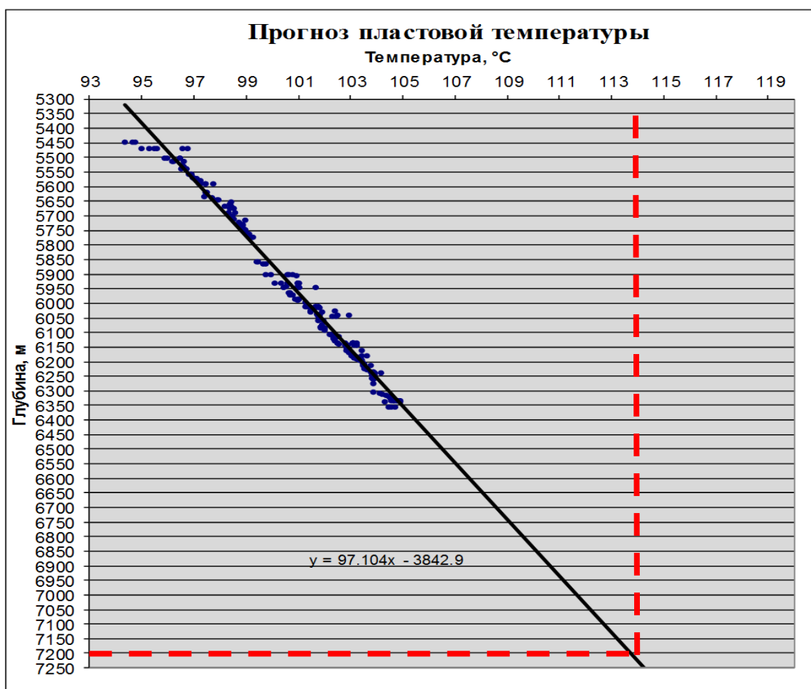
Figure 10 - Graph of temperature versus depth (temperature gradient) at Shah-Deniz
