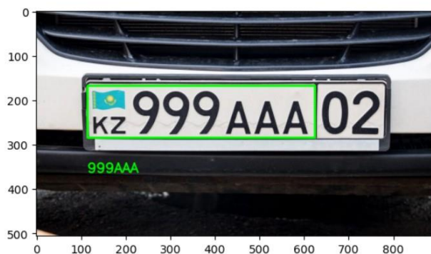
Fig.4. Visualization of text and region of number plate on image
