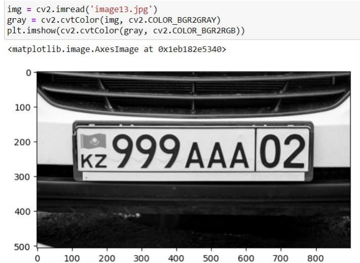
Fig. 1. Reading image and grayscale conversion
