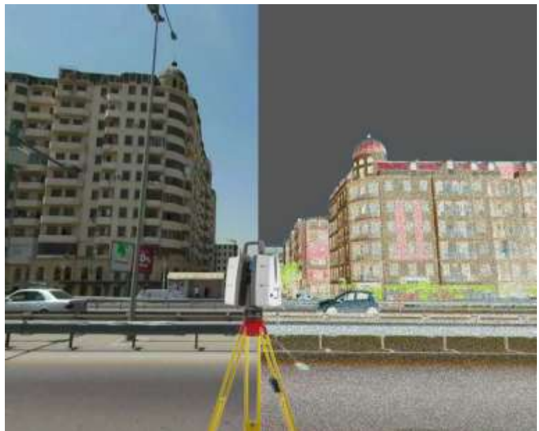
Figure 3. Scanning an area using a terrestrial laser
