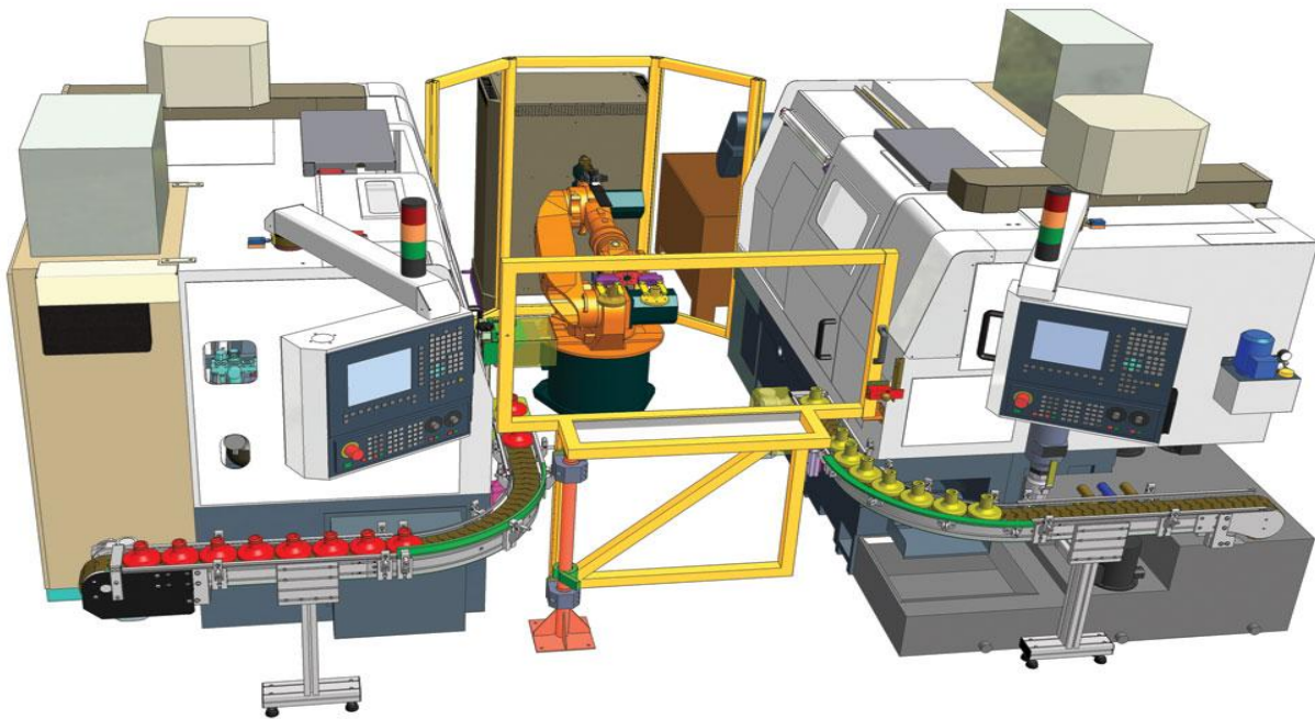
Figure 1. Automated CNC Machine Tool System and Robot-Manipulator Manufacturing Cell
